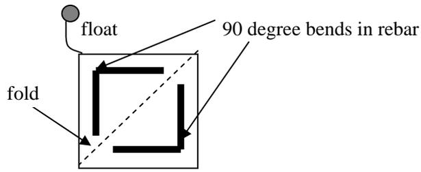
This small (5' x 5') benthic mat can fold diagonally for easier deployment and positioning by one person on uneven substrate. The rebar sections are not connected to each other at two of the corners, allowing the barrier to be folded. A float is attached at one corner to help locate the mat.
